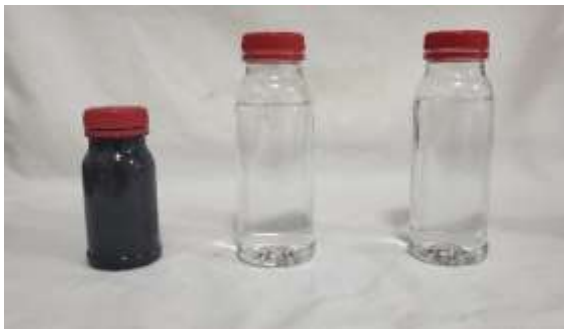
Process water from a smeltery, before (the sample to the left) and after (samples in the middle and to the right) purification with AxoPur.
